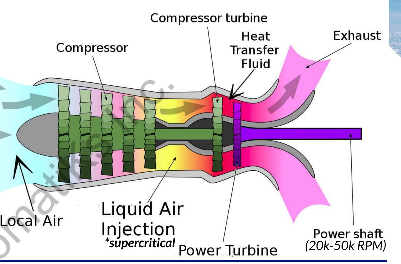
Increasing shaft RPM <u>2x</u> increases power output <u>2x</u> with the same <u>size and mass</u> of generator
